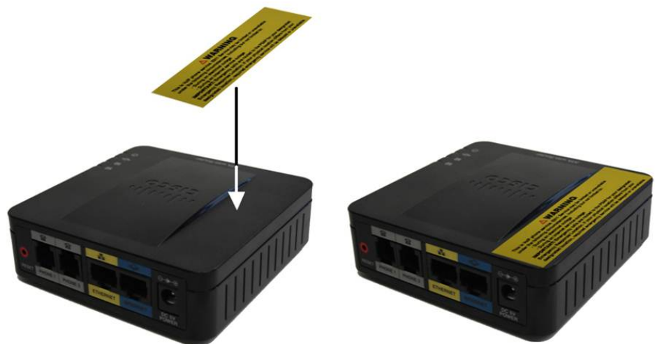
E911 Service WARNING Sticker
